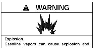
severe injury or death. Before starting generator set, operate blower 4 minutes and check engine compartment for
